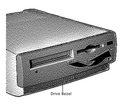
4 Swing up the drive bezel and pull it away from the metal chassis.
