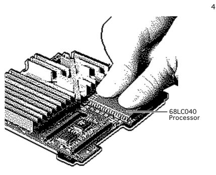
**Caution:** Forcing the 68LC040 processor connector pins into the socket could damage the pins. If the processor resists installation, check the pin alignment.
