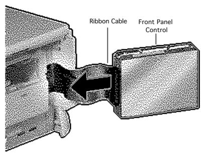
Disconnect the front panel control from the ribbon cable.
