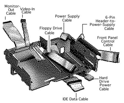
Replacement Note: Arrange the cables as shown before replacing the shield/wiring harness. When dressing the cables, do not crimp them between the harness and the floor of the bottom case, or between the harness and the sides of the bottom case. Route the speaker cable between the logic board connector and the CD-ROM shelf. Route front panel control, power supply, and header cables to the side of the front panel control bay.
