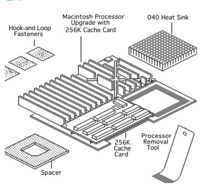
The upgrade board includes the PowerPC 601 processor on board and a socket to accept the customer's 68LC040 processor.
