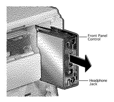
Pull the front panel control out just far enough to reach the ribbon cable connector.
