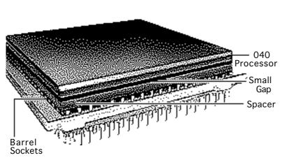
Note: On a correctly installed 040 processor, a very small gap separates the 040 chip from the metal spacer. A larger gap caused by the barrel sockets of the upgrade board separates the upgrade board and the spacer.
